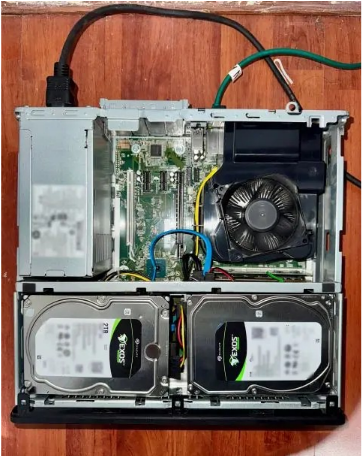
Figure 1. Sanitised view of the completed internal NAS hardware layout.
